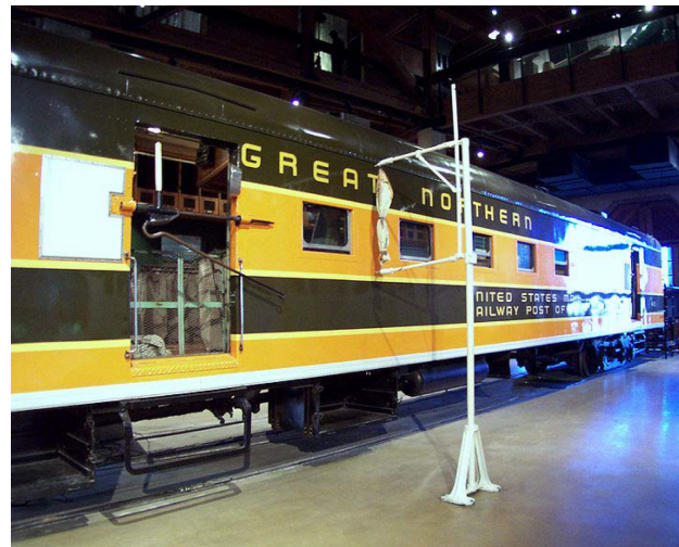
Fig. 2. A Great Northern RR mail car showing the mail catcher system: an arm extending from the open door of the mail car which catches the mail bag hung between the two horizontal arms of the white trackside stanchion.
